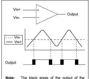
te: The black areas of the output of the comparator represents the uncertainty due to input offsets and response time.
