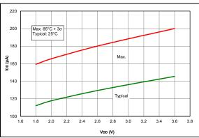
FIGURE 36-3: IDD, EC Oscillator LP Mode, Fosc = 500 kHz, PIC16LF1614/8 Only.
