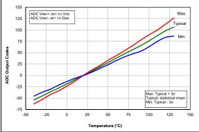
FIGURE 36-76: Temp. Indicator Slope Normalized to 20°C, Low Range, VDD = 3.0V, PIC16F1614/8 Only.
