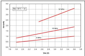
FIGURE 36-18: IDD Maximum, HFINTOSC Mode, PIC16LF1614/8 Only.
