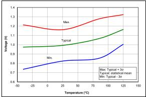
FIGURE 36-59: POR Rearm Voltage, NP Mode, PIC16LF1614/8 Only.
