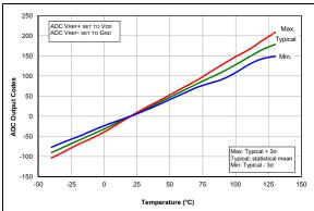
FIGURE 36-75: Temp. Indicator Slope Normalized to 20°C, High Range, VDD = 3.0V, PIC16F1614/8 Only.
