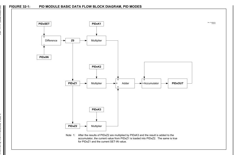
Within the controller, the input is subtracted from a preprogrammed set point to get an error value. This error value, along with the previous two error values (if any), are multiplied by user-input coefficients and the results of these multiplications are added together to make up the output. If the MODE<2:0> bits of the PIDxCON register = 101, the PID output is equal to the current output added to any previous outputs.
