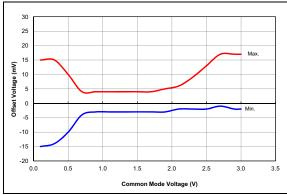
FIGURE 36-81: Comparator Offset, NP Mode (CxSP = 1), VDD = 3.0V, Typical Measured Values at 25°C.
