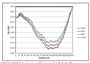
FIGURE 36-93: Typical DAC INL Error, VDD = 5.0V, VREF = External 5V, PIC16F1614/8 Only.
