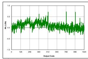
FIGURE 36-65: ADC 10-bit Mode, Single-Ended INL, VDD = 3.0V, TAD = 1  $\mu$ S, 25°C.
