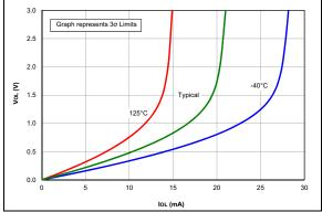
FIGURE 36-40: VOL vs. IOL Over Temperature, VDD = 3.0V.
