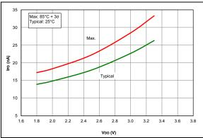
FIGURE 36-23: IPD, Fixed Voltage Reference (FVR), PIC16LF1614/8 Only.
