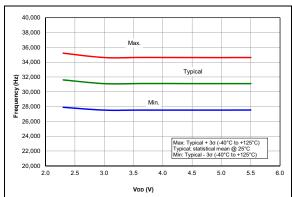
FIGURE 36-44: LFINTOSC Frequency, PIC16F1614/8 Only.
