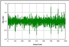
FIGURE 36-63: ADC 10-bit Mode, Single-Ended DNL, VDD = 3.0V,  $TAD = 1 \mu S$ ,  $25^{\circ}C$ .
