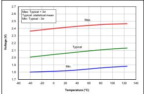
FIGURE 36-53: LPBOR Reset Voltage.
