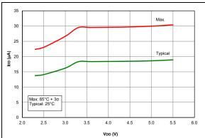
FIGURE 36-2: IDD, EC Oscillator LP Mode, Fosc = 32 kHz, PIC16F1614/8 Only.
