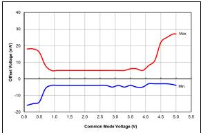
FIGURE 36-85: Comparator Offset, NP Mode (CxSP = 1), VDD = 5.5V, Typical Measured Values From -40°C to 125°C, PIC16F1614/8 Only.
