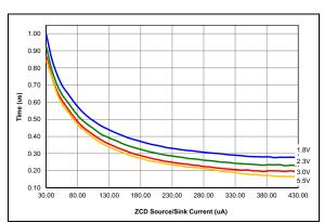
FIGURE 36-102: ZCD Pin Response Timer over Current, Typical Measured Values from -40°C to 125°C.
