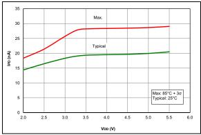
FIGURE 36-24: IPD, Fixed Voltage Reference (FVR), PIC16F1614/8 Only.
