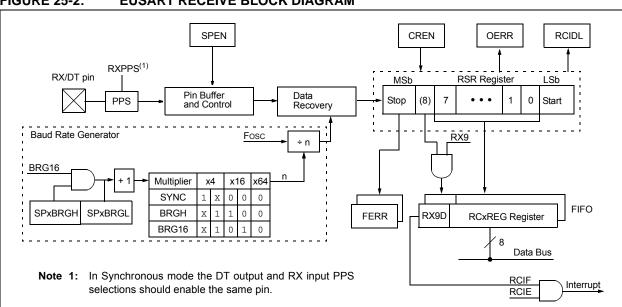
FIGURE 25-2: EUSART RECEIVE BLOCK DIAGRAM
