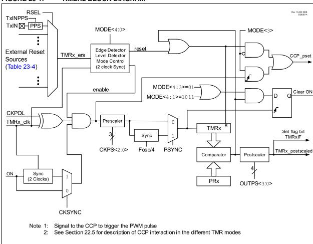
FIGURE 23-2: TIMER2 CLOCK SOURCE BLOCK DIAGRAM
