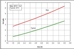
FIGURE 36-29: IPD, Timer1 Oscillator, Fosc = 32 kHz, PIC16LF1614/8 Only.
