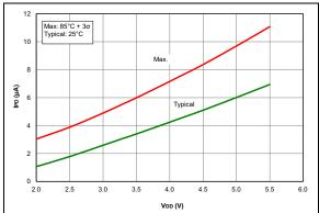
FIGURE 36-30: IPD, Timer1 Oscillator, Fosc = 32 kHz, PIC16F1614/8 Only.
