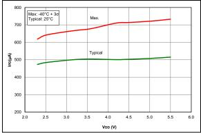
**FIGURE 36-34:** IPD, Comparator, NP Mode (CxSP = 1), PIC16F1614/8 Only.
