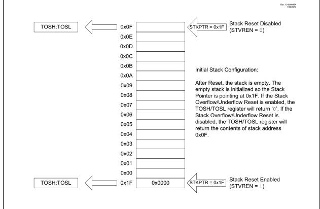
FIGURE 3-5: ACCESSING THE STACK EXAMPLE 2
