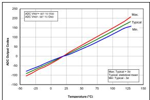
FIGURE 36-79: Temp. Indicator Slope
