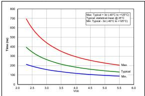
FIGURE 36-89: Comparator Output Filter
