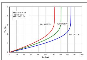
**FIGURE 36-38:** VOL vs. IOL Over Temperature for High Drive Pins, VDD = 5.0V, PIC16F1614/8 Only.
