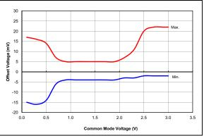
**FIGURE 36-82:** Comparator Offset, NP Mode (CxSP = 1), VDD = 3.0V, Typical Measured Values From -40°C to 125°C.
