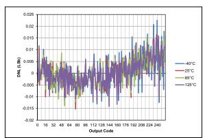
FIGURE 36-90: Typical DAC DNL Error, VDD = 3.0V, VREF = External 3V.
