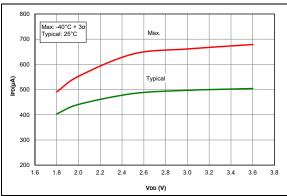
**FIGURE 36-33:** IPD, Comparator, NP Mode (CxSP = 1), PIC16LF1614/8 Only.
