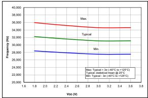
FIGURE 36-43: LFINTOSC Frequency, PIC16LF1614/8 Only.
