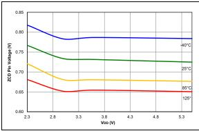
FIGURE 36-99: ZCD Pin Voltage, Typical Measured Values.
