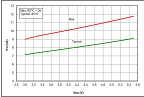
**FIGURE 36-26:** IPD, Brown-Out Reset (BOR), BORV = 1, PIC16F1614/8 Only.
