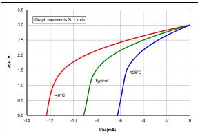
FIGURE 36-39: VOH vs. IOH Over Temperature, VDD = 3.0V.
