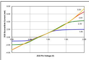
FIGURE 36-101: ZCD Pin Current over ZCD Pin Voltage, Typical Measured Values from -40°C to 125°C.
