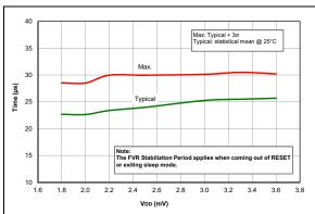
**FIGURE 36-62:** FVR Stabilization Period, PIC16LF1614/8 Only.
