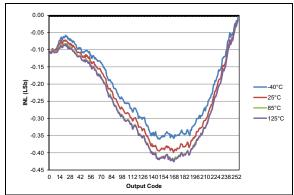
FIGURE 36-91: Typical DAC INL Error, VDD = 3.0V, VREF = External 3V.
