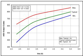
FIGURE 36-72: Temp. Indicator Initial Offset, Low Range, Temp. = 20°C, PIC16F1614/8 Only.
