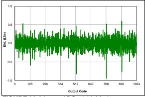
**FIGURE 36-64:** ADC 10-bit Mode, Single-Ended DNL, VDD = 3.0V,  $TAD = 4 \mu S$ ,  $25^{\circ}C$ .
