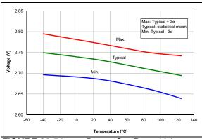
**FIGURE 36-51:** Brown-Out Reset Voltage, High Trip Point (BORV = 0).
