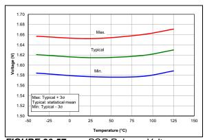
FIGURE 36-57: POR Release Voltage.
