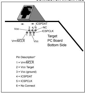
Another connector often found in use with the PICkit™ programmers is a standard 6-pin header with 0.1 inch spacing. Refer to Figure 33-2.
