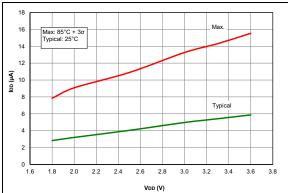
FIGURE 36-1: IDD, EC Oscillator LP Mode, Fosc = 32 kHz, PIC16LF1614/8 Only.
