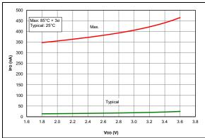
FIGURE 36-31: IPD, ADC Non-Converting, PIC16LF1614/8 Only.
