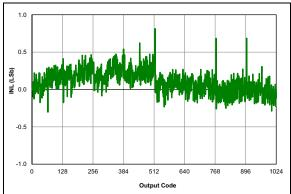
**FIGURE 36-66:** ADC 10-bit Mode, Single-Ended INL, VDD = 3.0V, TAD =  $4 \mu$ S, 25°C.
