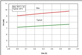
**FIGURE 36-25:** IPD, Brown-Out Reset (BOR), BORV = 1, PIC16LF1614/8 Only.
