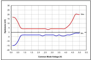
FIGURE 36-84: Comparator Offset, NP Mode (CxSP = 1), VDD = 5.0V, Typical Measured Values at 25°C, PIC16F1614/8 Only.
