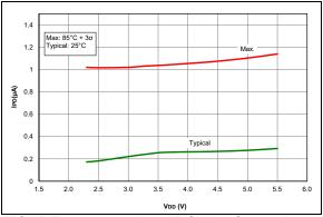
FIGURE 36-32: IPD, ADC Non-Converting, PIC16F1614/8 Only.
