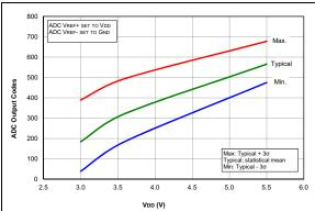
FIGURE 36-71: Temp. Indicator Initial Offset, High Range, Temp. = 20°C, PIC16F1614/8 Only.
