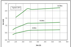
FIGURE 36-19: IDD Typical, HFINTOSC Mode, PIC16F1614/8 Only.
