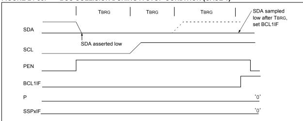
FIGURE 24-39: BUS COLLISION DURING A STOP CONDITION (CASE 2)
