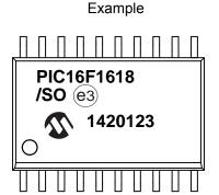
20-Lead SSOP (5.30 mm)
