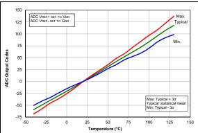
FIGURE 36-74: Temp. Indicator Slope Normalized to 20°C, High Range, VDD = 5.5V, PIC16F1614/8 Only.
