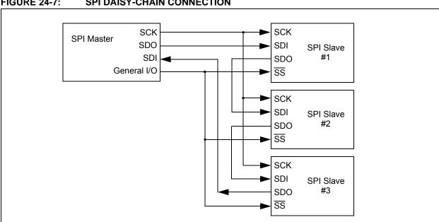
**FIGURE 24-7: SPI DAISY-CHAIN CONNECTION**
