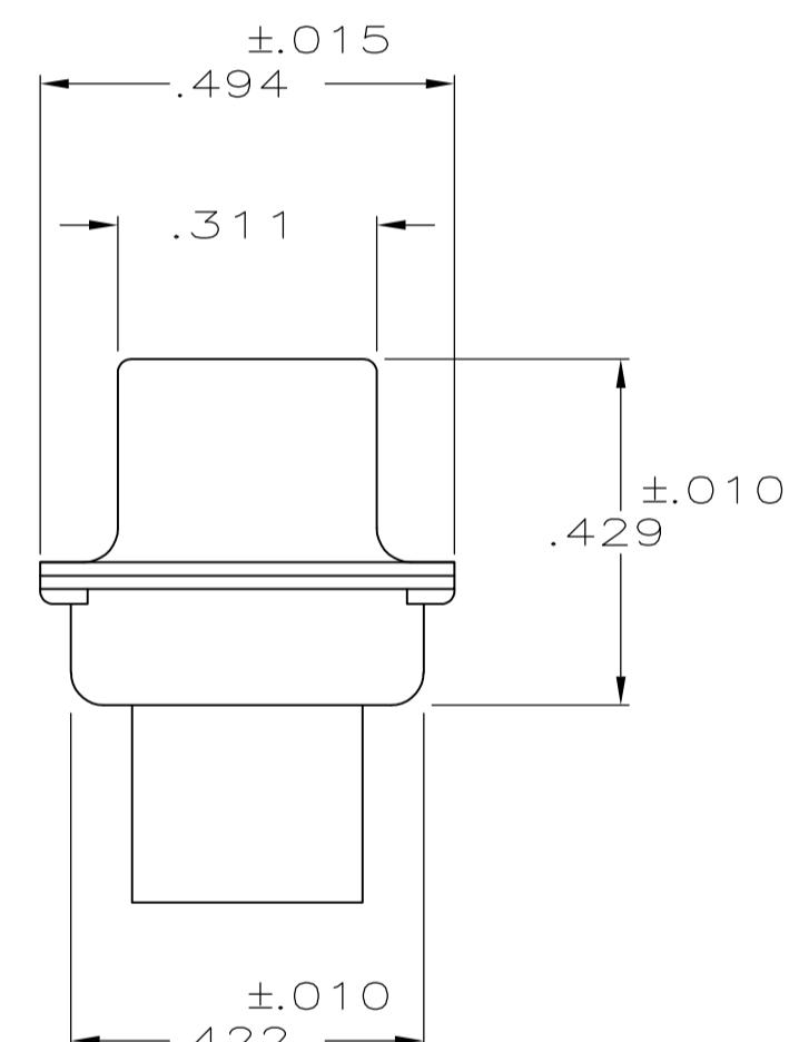
1. THIS RECEPTACLE WILL MATE WITH ANY SIZE 3,44 POSN. PLUG IN AMPLIMITE SERIES.
