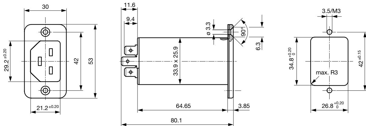
Screw-on mounting with wire leads
