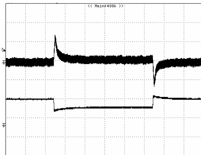
Figure 9: Output voltage response to step-change in load current (75%-50%-75% of I_o , max; di/dt = 2.5A/\mu s ). Load cap: 330\mu F , 35m\Omega ESR solid electrolytic capacitor and 1\mu F ceramic capacitor. Top Trace: V_{out} (100mV/div, 200us/div), Bottom Trace: I_{out} (5A/div). Scope measurement should be made using a BNC cable (length shorter than 20 inches). Position the load between 51 mm to 76 mm (2 inches to 3 inches) from the module.
