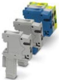
Plug, Connection method: Spring-cage connection, Number of positions: 1, Cross section: 0.08 mm<sup>2</sup> - 4 mm<sup>2</sup>, AWG: 28 - 12, Width: 5.2 mm, Height: 34 mm, Color: green-yellow
