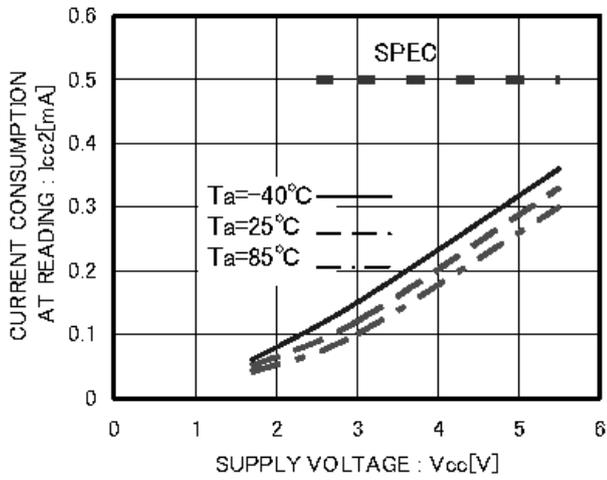
Figure 10. Current consumption at READ operation
