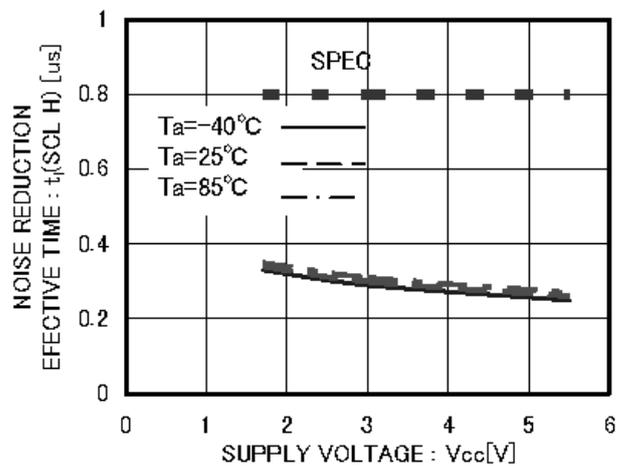
Figure 25. Noise reduction affection time t(SCL H)
