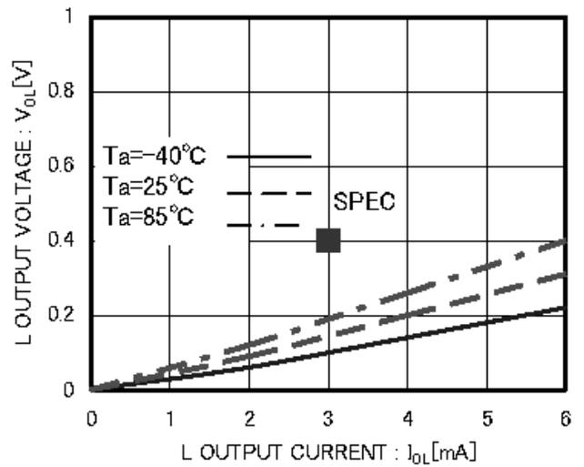
Figure 5. "L" Output Voltage  $V_{OL}$ - $I_{OL}$
