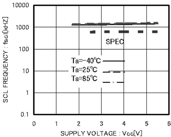
Figure 12. SCL frequency f<sub>SCL</sub>
