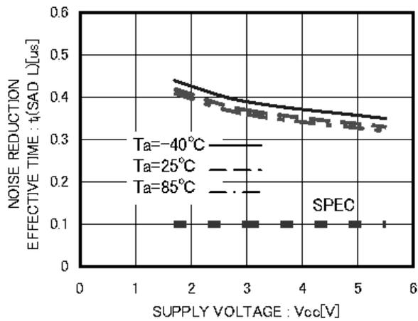
Figure 28. Noise reduction effective time  $t_I(SDA L)$
