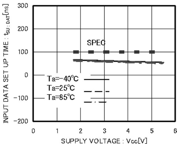
Figure 20. Input Data Setup Time  $t_{SU:DAT}(LOW)$
