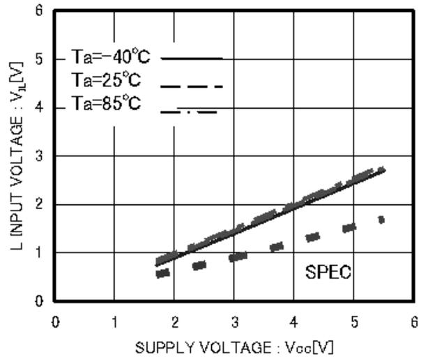
Figure 3. "L" Input Voltage  $V_{IL}$
