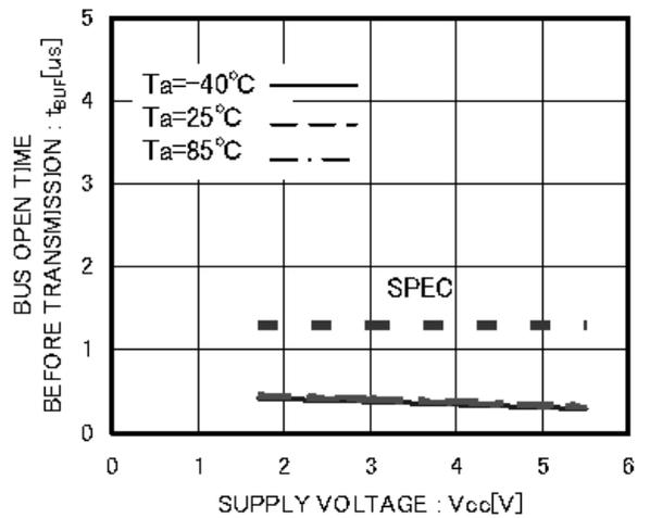
Figure 23. BUS open time before transmission tBUF
