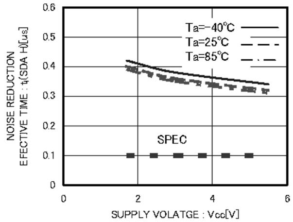
Figure 27. Noise reduction effective time  $t_I(SDA H)$
