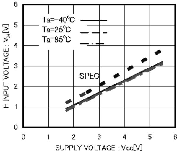
Figure 2. "H" Input Voltage  $V_{IH}$
