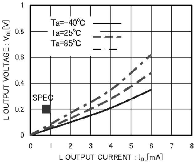
Figure 4. "L" Output Voltage  $V_{OL}$ - $I_{OL1}$
