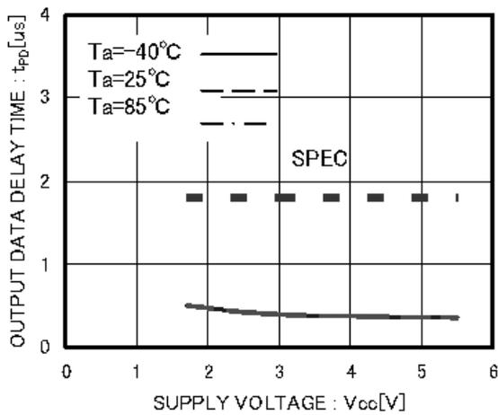
Figure 22. "H" Data output delay time tPD1
