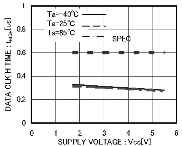
Figure 13. Data clock High Period t<sub>HIGH</sub>
