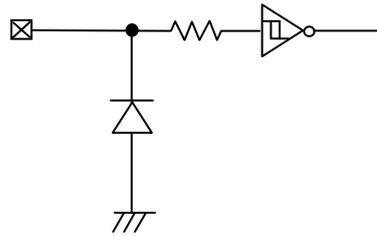
Figure 53. Input pin circuit diagram
