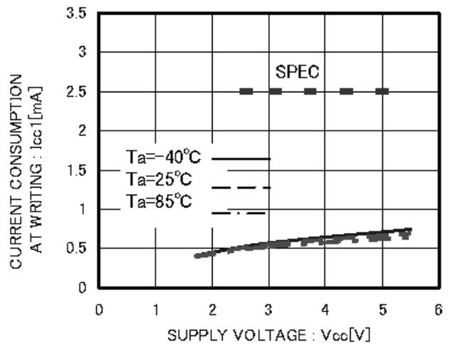
Figure 9. Current consumption at WRITE operation
