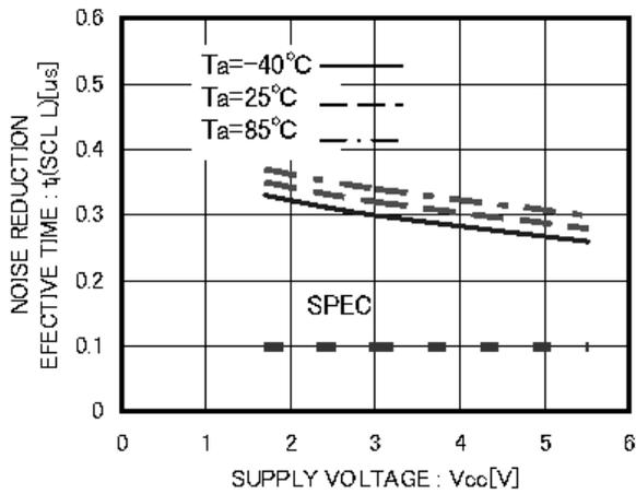
Figure 26. Noise reduction effective time  $t_I(SCL L)$
