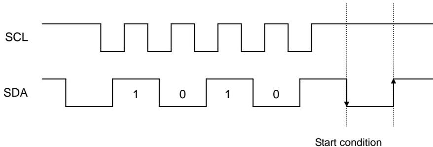
Figure 47. Case of cancel by start, stop condition during slave address input
