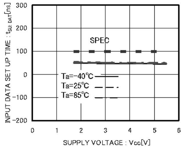
Figure 19. Input Data Setup Time  $t_{SU:DAT}(HIGH)$
