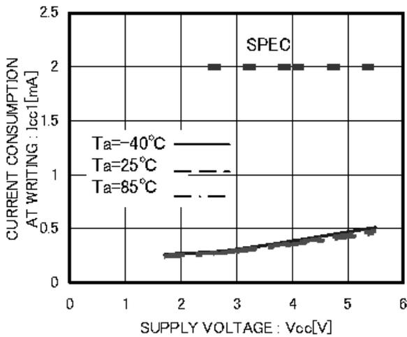
Figure 8. Current consumption at WRITE operation
