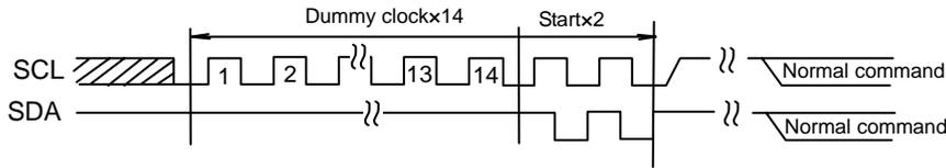
Figure 44-(a) The case of 14 Dummy clock + START + START+ command input
