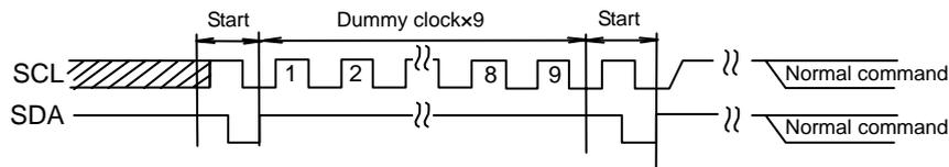
Figure 44-(b) The case of START+9 Dummy clock + START + command
