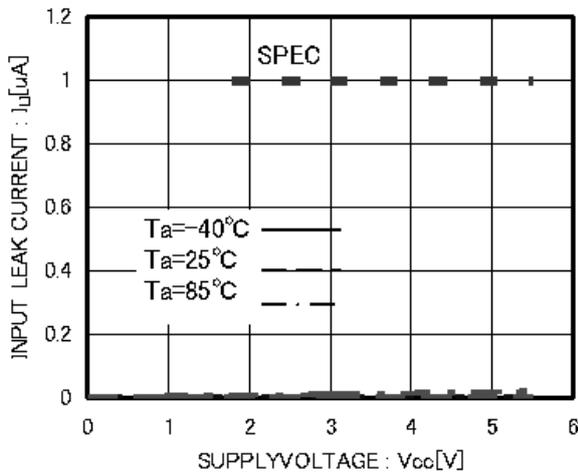
Figure 6. Input Leak Current Ili
