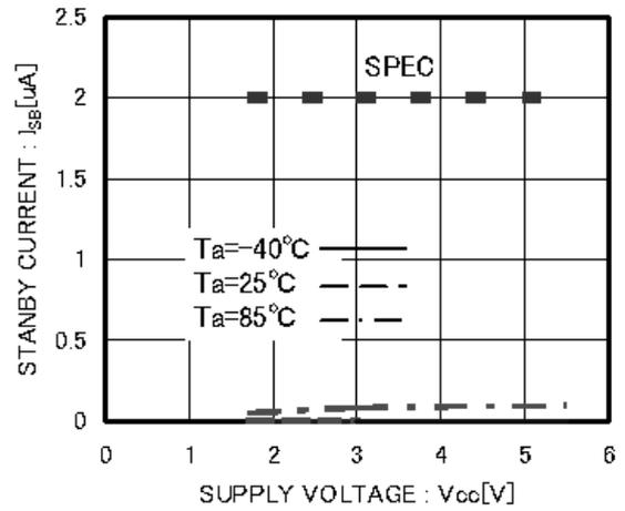
Figure 11. Standby operation I<sub>SB</sub>
