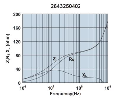
Impedance, reactance, and resistance vs. frequency.
