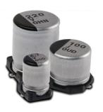
Type AVES Capacitors are rated for 1000 hours at 105 °C with low impedance characteristics. They are ideal for high density PC board packaging. The Type AVES offers a low in-place-cost for a high quality performer. The vertical cylindrical cases facilitate automatic mounting and reflow soldering into the same footprint of like-rated tantalum capacitors except without the need for voltage derating.
