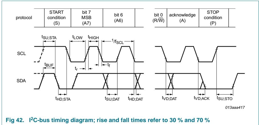
Fig 42. I<sup>2</sup>C-bus timing diagram; rise and fall times refer to 30 % and 70 %
