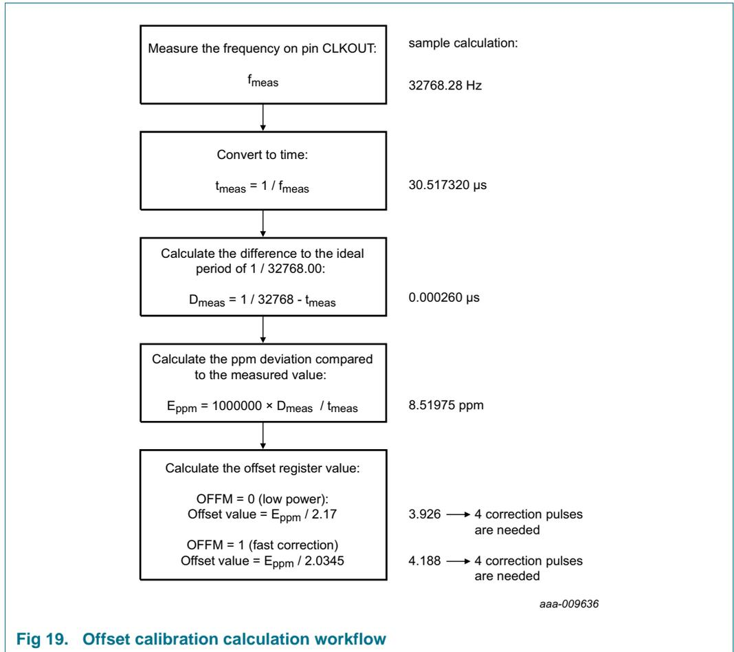
Fig 19. Offset calibration calculation workflow
