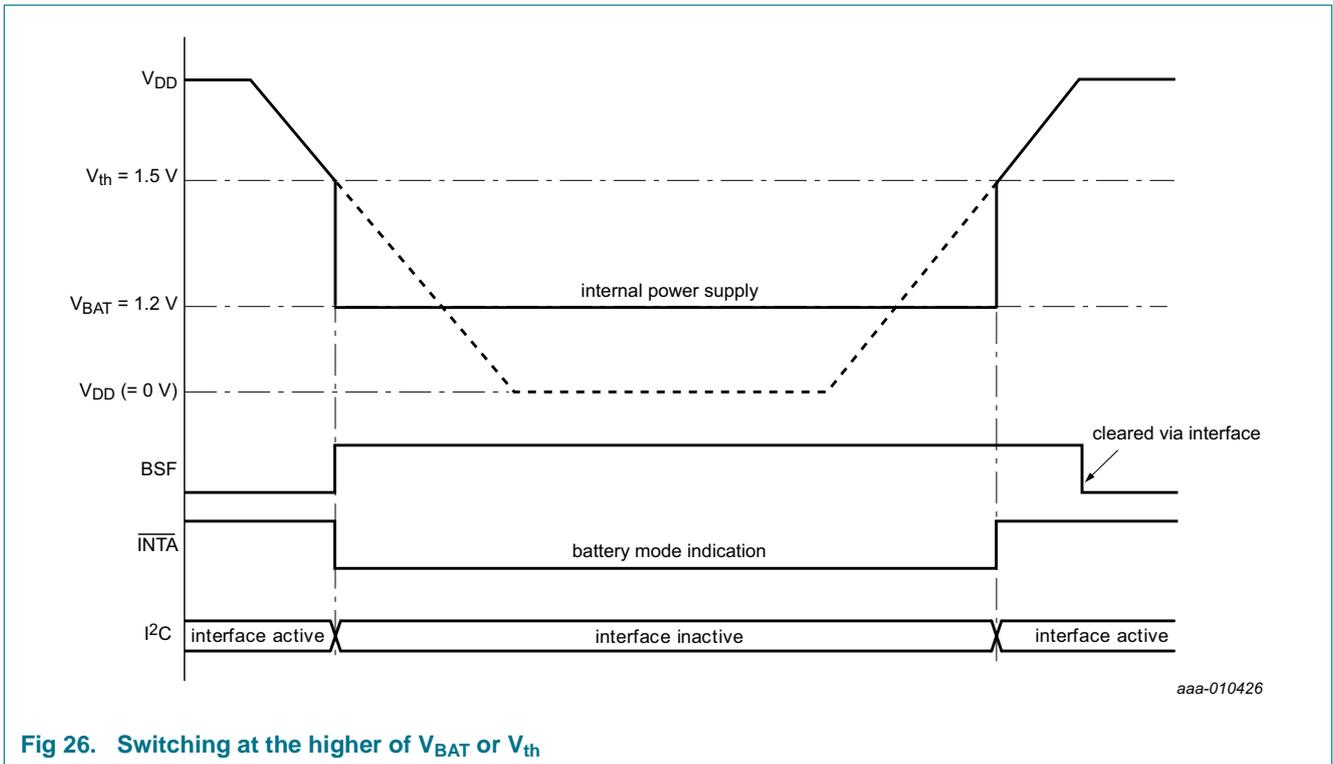
Fig 26. Switching at the higher of V<sub>BAT</sub> or V<sub>th</sub>
