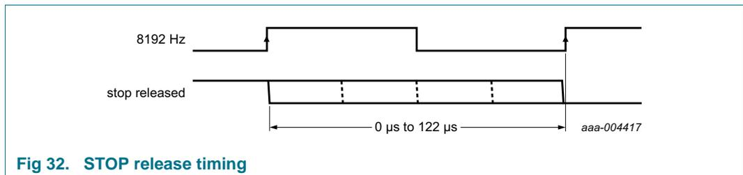
The first increment of the time circuits is between 0 s and 122 μs after STOP is released.
