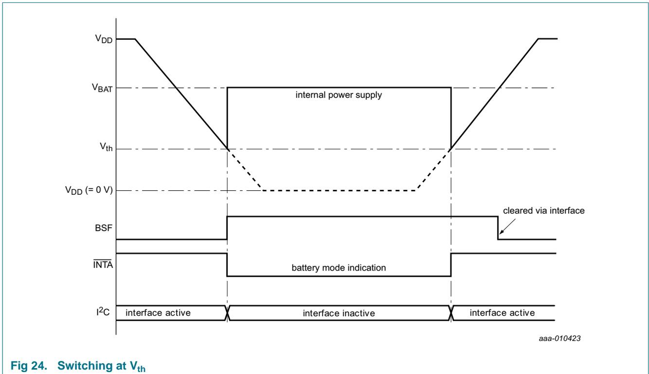
Fig 24. Switching at V<sub>th</sub>
