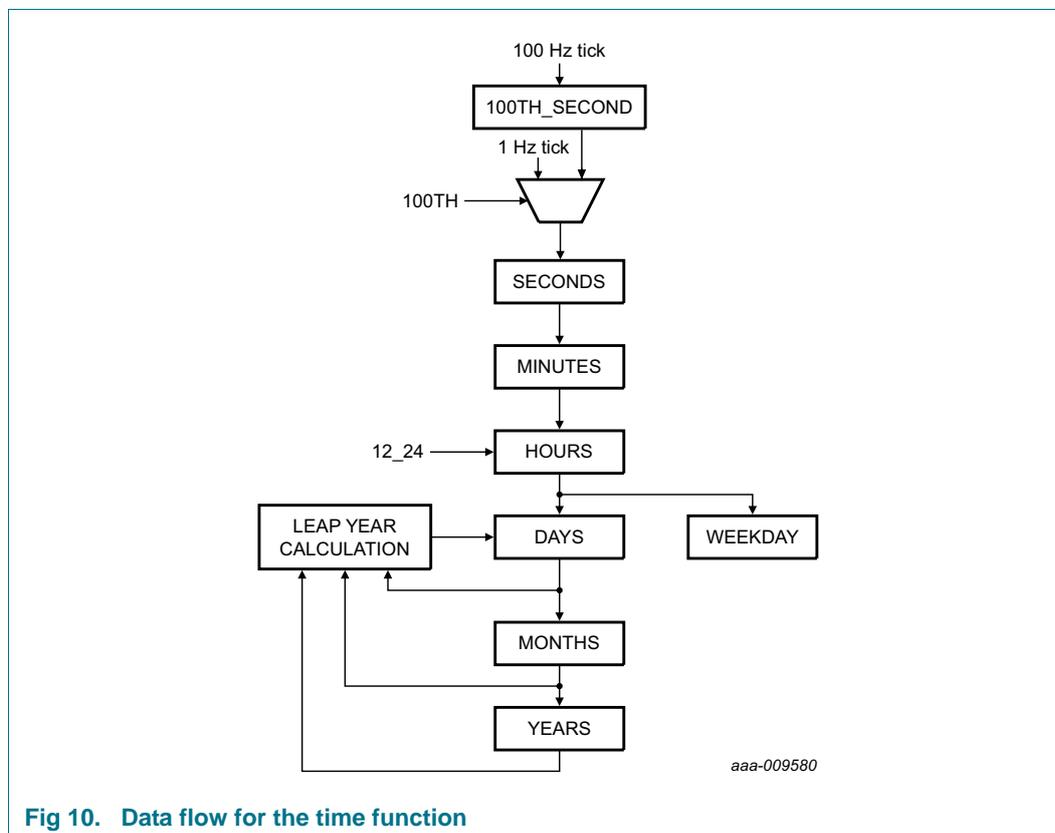
Fig 10. Data flow for the time function
