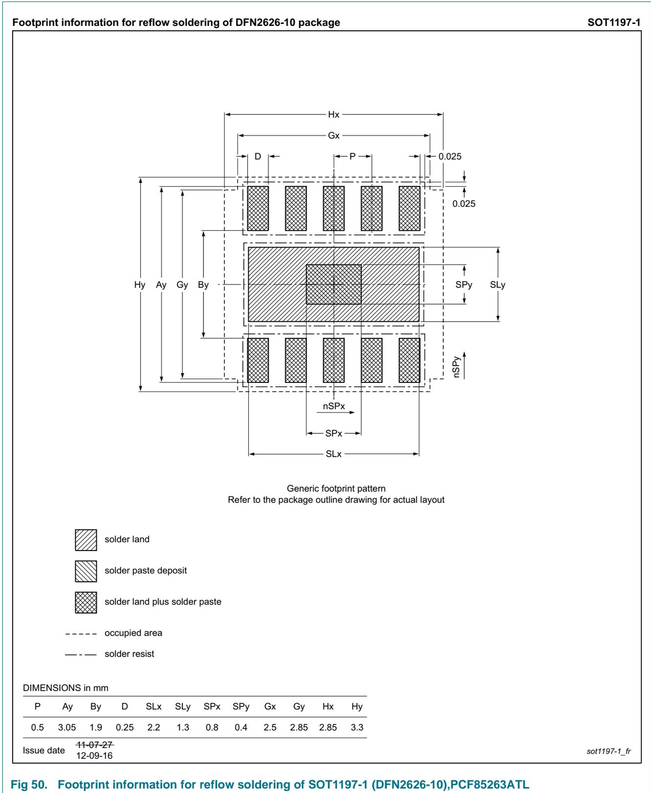
**Fig 50. Footprint information for reflow soldering of SOT1197-1 (DFN2626-10),PCF85263ATL**
