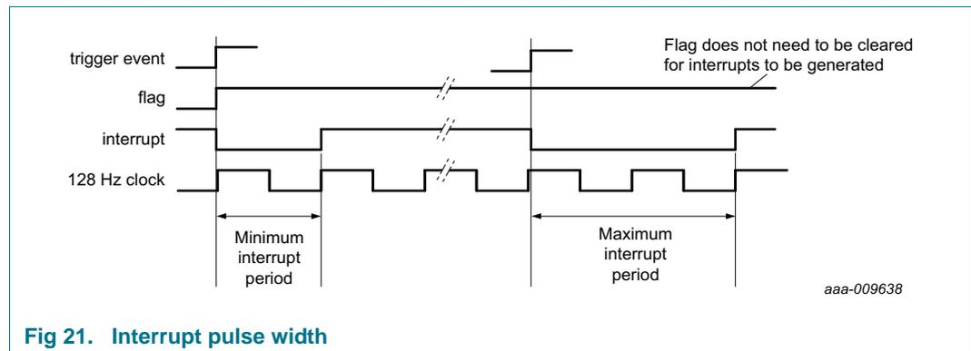
**Fig 21. Interrupt pulse width**
