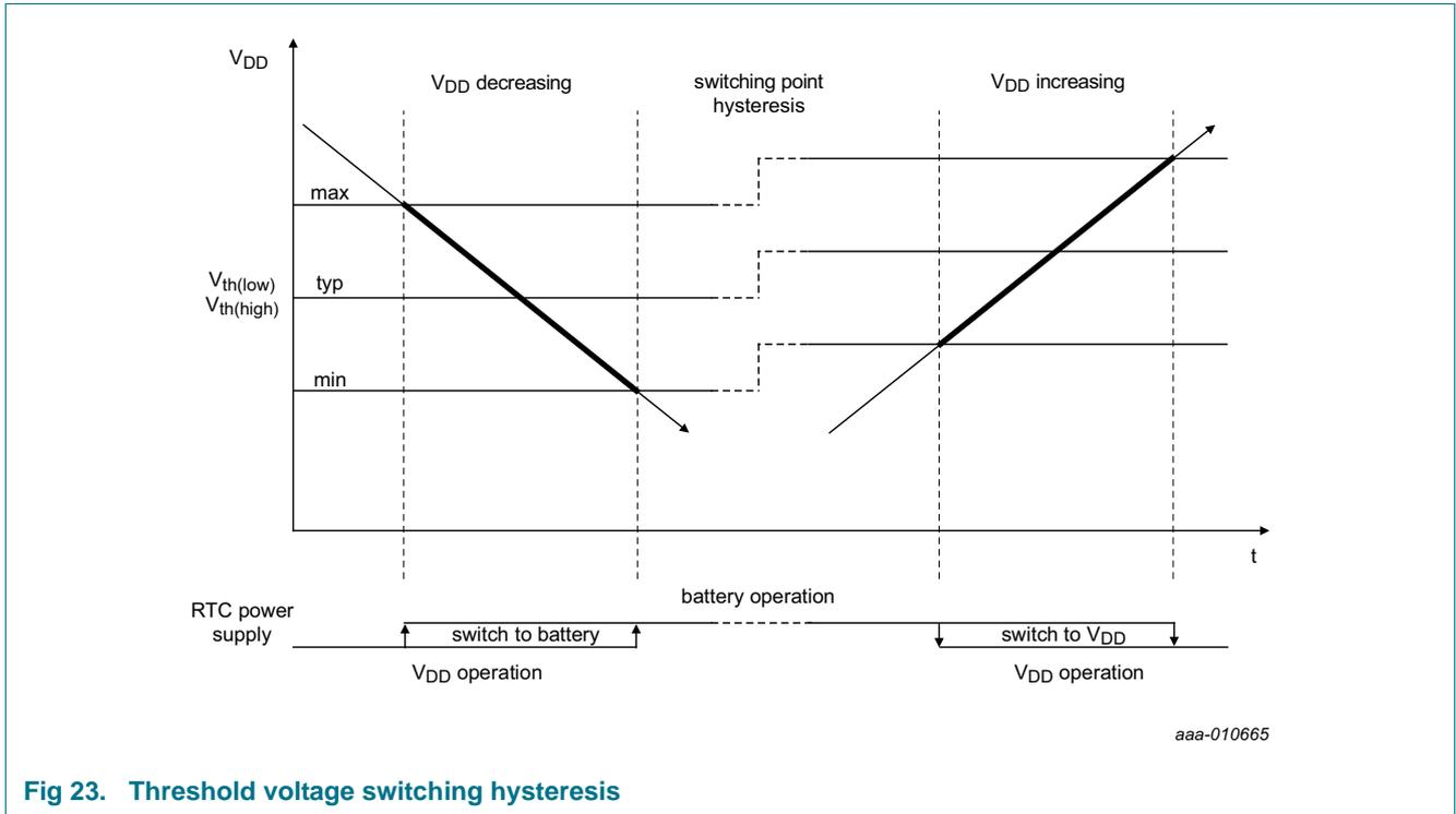
Fig 23. Threshold voltage switching hysteresis
