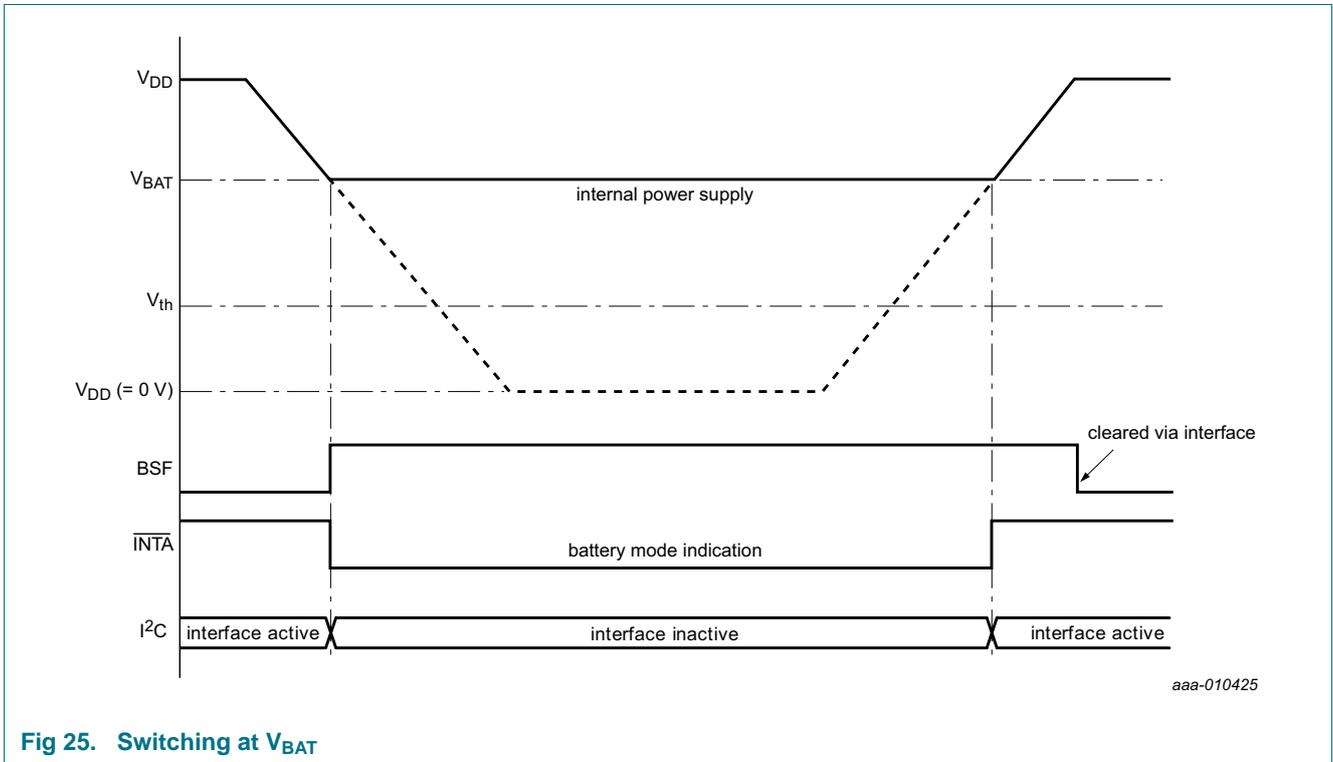
Fig 25. Switching at V<sub>BAT</sub>
