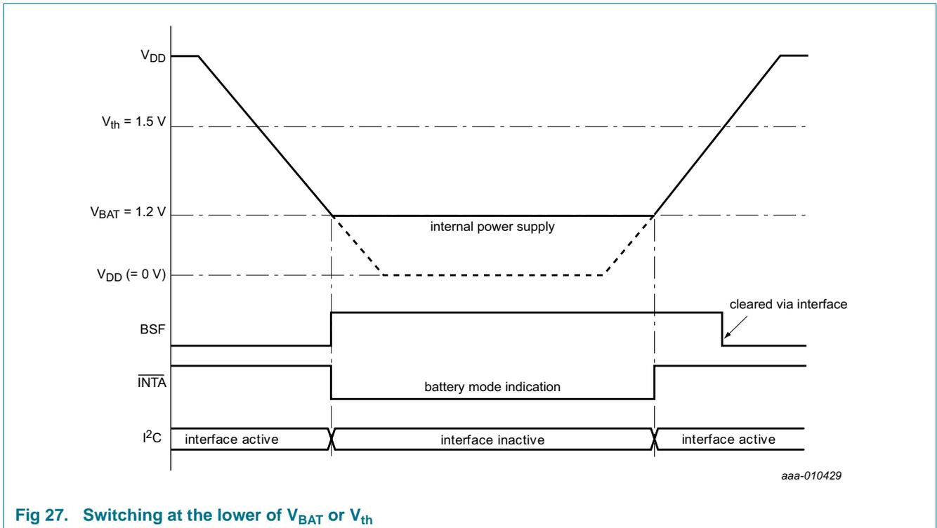
Fig 27. Switching at the lower of V<sub>BAT</sub> or V<sub>th</sub>
