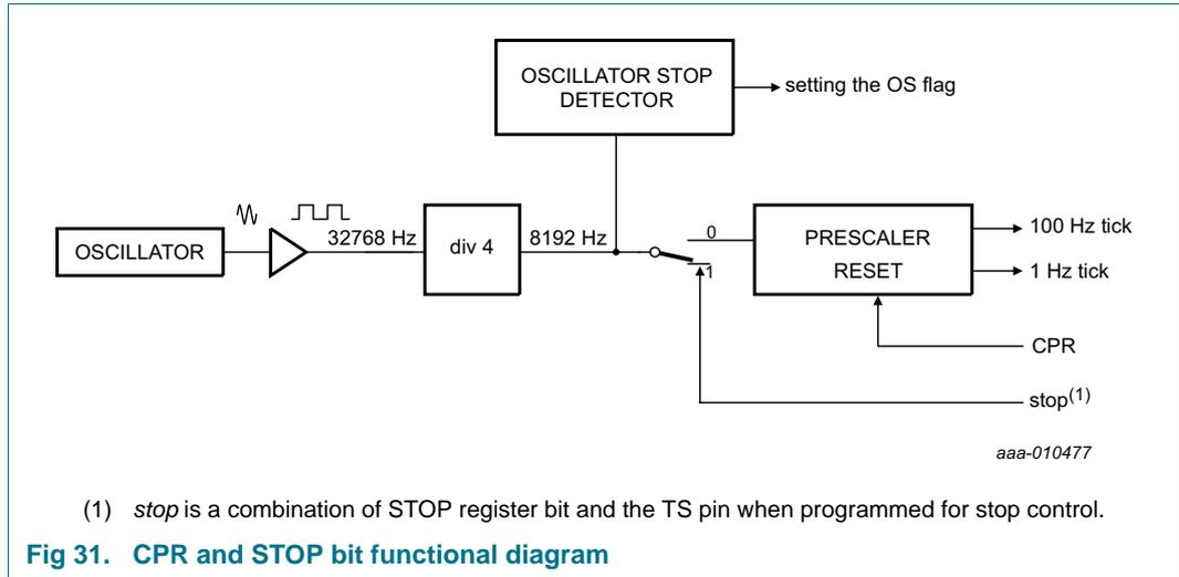
The *stop* signal blocks the 8.192 kHz clock from generating system clocks and freezes the time. In this state, the prescaler can be cleared with the CPR command in the Resets register (Section 8.15 on page 58).
