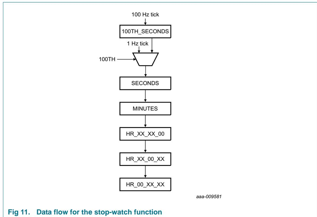
Fig 11. Data flow for the stop-watch function
