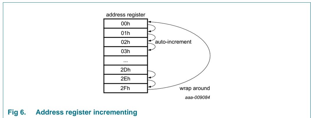
**Fig 6. Address register incrementing**
