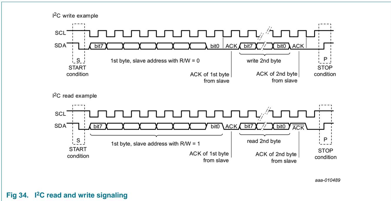
Fig 34. I<sup>2</sup>C read and write signaling
