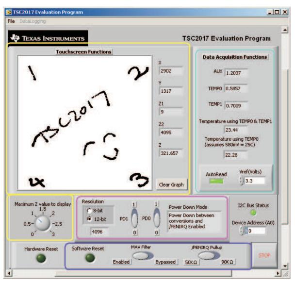
Figure 3. Four Main Sections in TSC2017EVM-PDK GUI Screen
