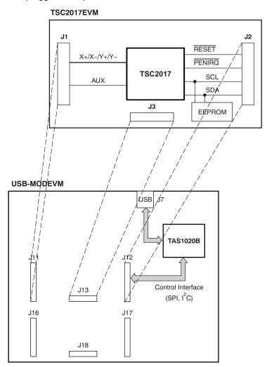
Figure 1. TSC2017EVM-PDK Hardware Block Diagram and Connection
