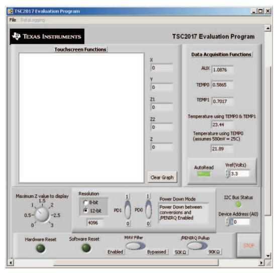
Figure 2. TSC2017EVM-PDK Software GUI Screen
