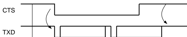
Figure 30-29. Transmitter Behavior when Operating with Hardware Handshaking
