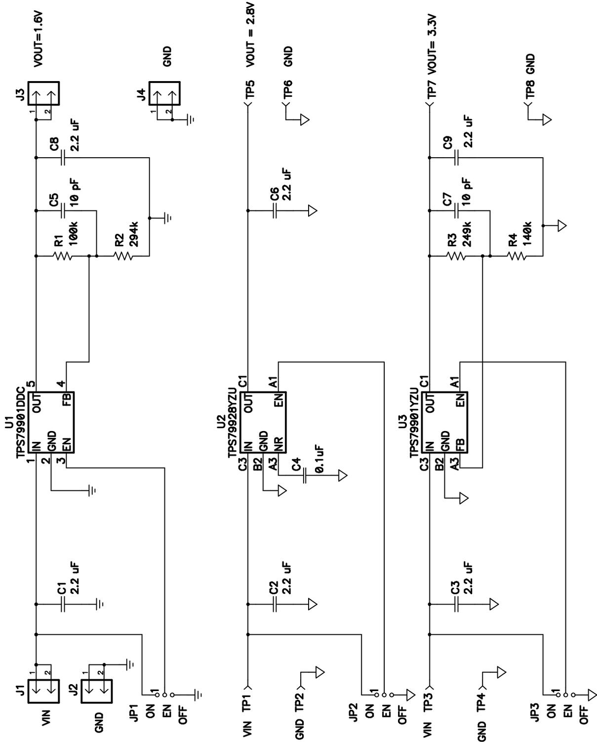
Figure 4. TPS799xxEVM-105 Schematic
