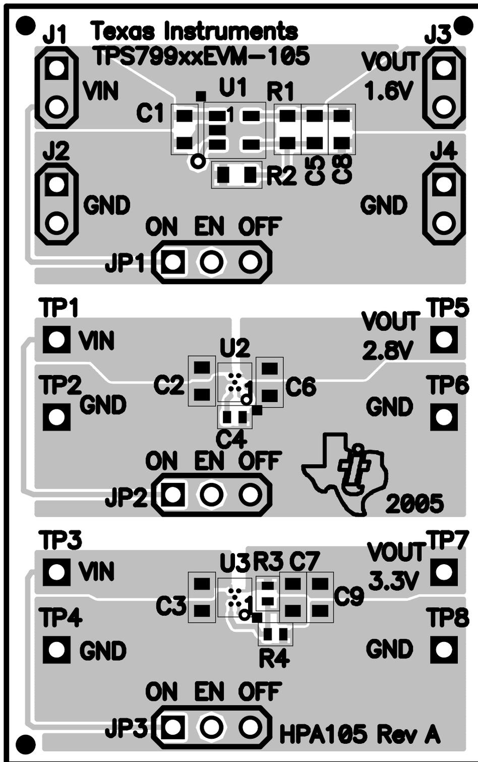
Figure 1. Assembly Layer
