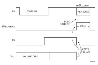
Figure 4. DC/DC Turn Off Blanking (LTC2950-1)
