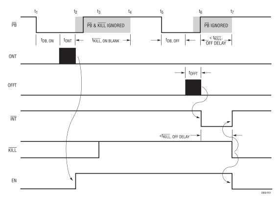
Figure 1. Simplified Power On/Off Sequence for LTC2950-1
