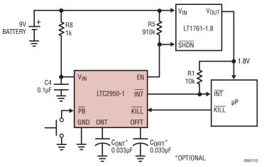
Figure 10. Reverse Battery Protection
