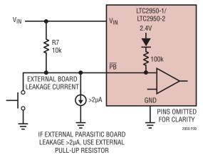
Figure 9. External Pull-Up Resistor on PB Pin
