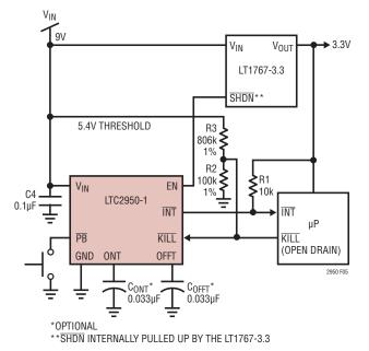
Figure 5. Input Voltage Monitoring with KILL Input
