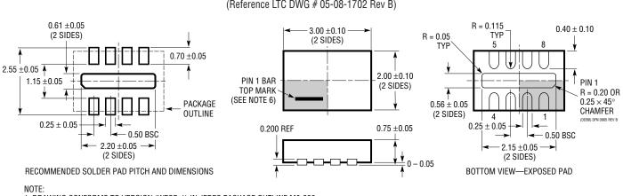
DDB Package 8-Lead Plastic DFN (3mm × 2mm) (Reference LTC DWG # 05-08-1702 Rev B)
