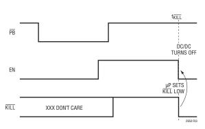
Figure 3.  $\mu$ P Turns Off Power (LTC2950-1)
