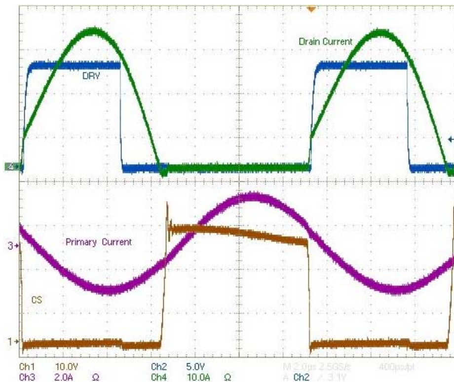
Figure 35. Waveforms from SR System Using MOSFET in TO220 Package without Parasitic Inductance Compensation – SR MOSFET Channel Conduction Time is Reduced
