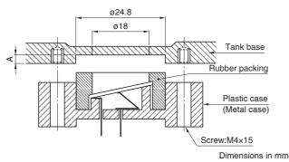
The transducer can beak off if the A dimension depth is shallow. TDK recommends a 2mm A-dimension depth and a screw tightening torque of  $0.39N \cdot m$ .
