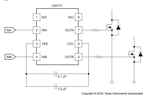
Figure 12. LM5111 Driving Two Independent MOSFETs
