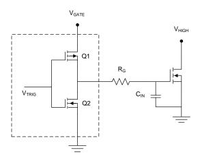
Figure 16. Driver Output Stage and Load
