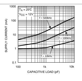
Figure 14. Supply Current vs Capacitive Load
