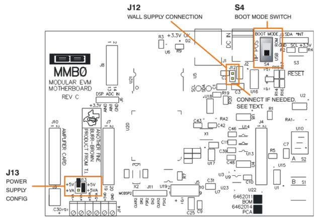
Figure 5. MMB0 Initial Setup
