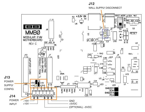
Figure 8. Using a External Supply For +5V
