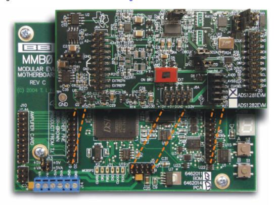
Figure 6. Connecting ADS1281EVM to MMB0
