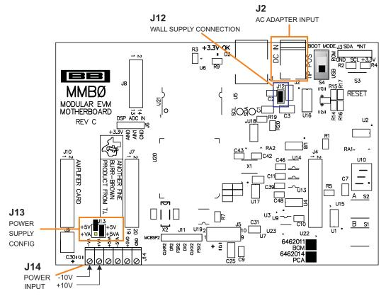
Figure 7. Using the +6V Wall Supply for +5V
