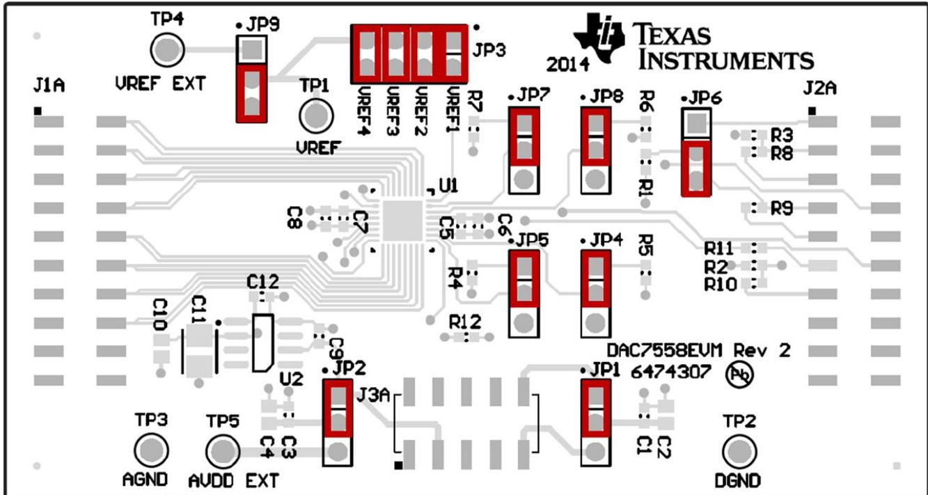
**Figure 1. Default Jumper Placement for the DAC7558EVM**
