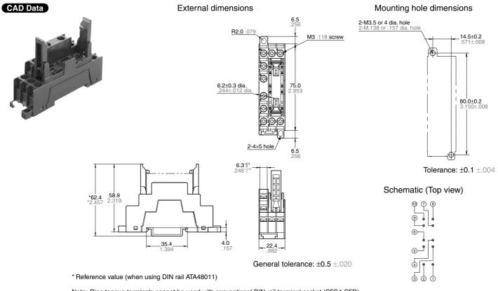
Note: Ring tongue terminals cannot be used with conventional DIN rail terminal socket (SFS4-SFD). In use of a ring tongue terminals, please use SFS4-SFD-R.
