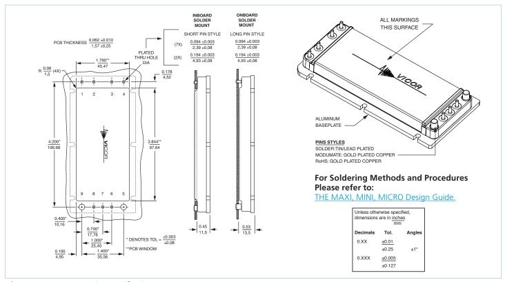
Figure 13 — PCB mounting specifications
