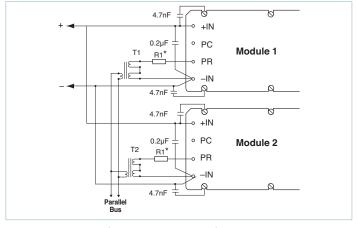
Figure 10 — Transformer-coupled interface
