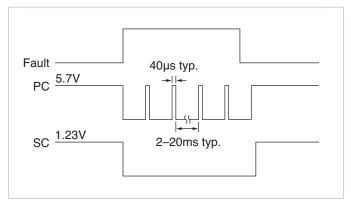
Figure 5 — PC/SC module alarm timing
