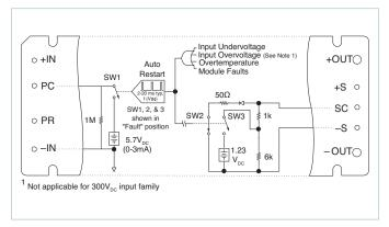
Figure 3 — PC/SC module alarm logic
