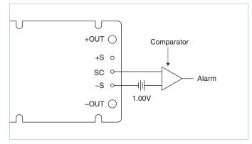
Figure 7 — Secondary side on-state indicator
