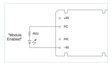
Figure 4 — LED on-state indicator
