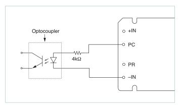
Figure 6 — Isolated on-state indicator
