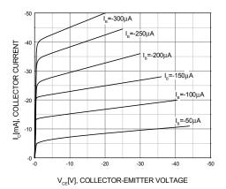
Figure 1. Static Characteristic
