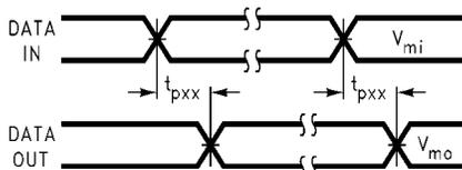
FIGURE 2. Waveform for Inverting and Non-Inverting Functions
