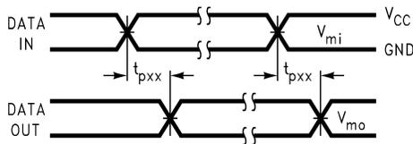
**FIGURE 8. Waveform for Inverting and Non-Inverting Functions**
