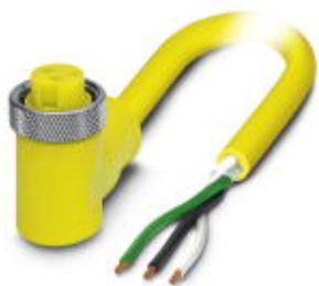
Sensor/actuator cable, 3-position, PVC, yellow, free cable end, on Socket angled 7/8"-16UNF, A-coded, cable length: 4 m
