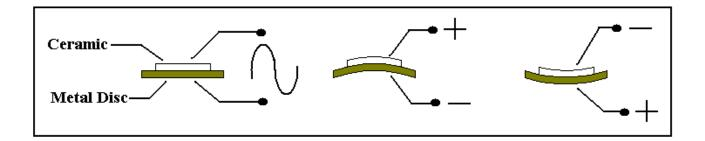
bonded to it that physically bends when voltage is applied to it.
