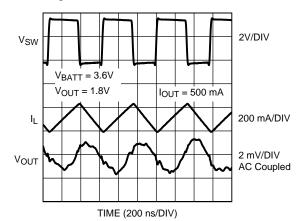
Figure 23. Typical PWM Operation
