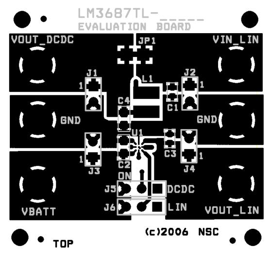
Figure 28. Top Layer Board Layout
