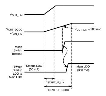
Figure 26. Startup Sequence,  $V_{EN_{DCDC}} = V_{EN_{LIN}} = V_{BATT}$
