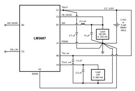
Figure 2. Typical Application Circuit: Independent Mode of Operation
