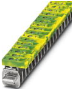
Connection terminal block, Connection method Screw connection, Cross section: 0.5 mm 2 - 6 mm 2 , Width: 7 mm, Color: green-yellow
