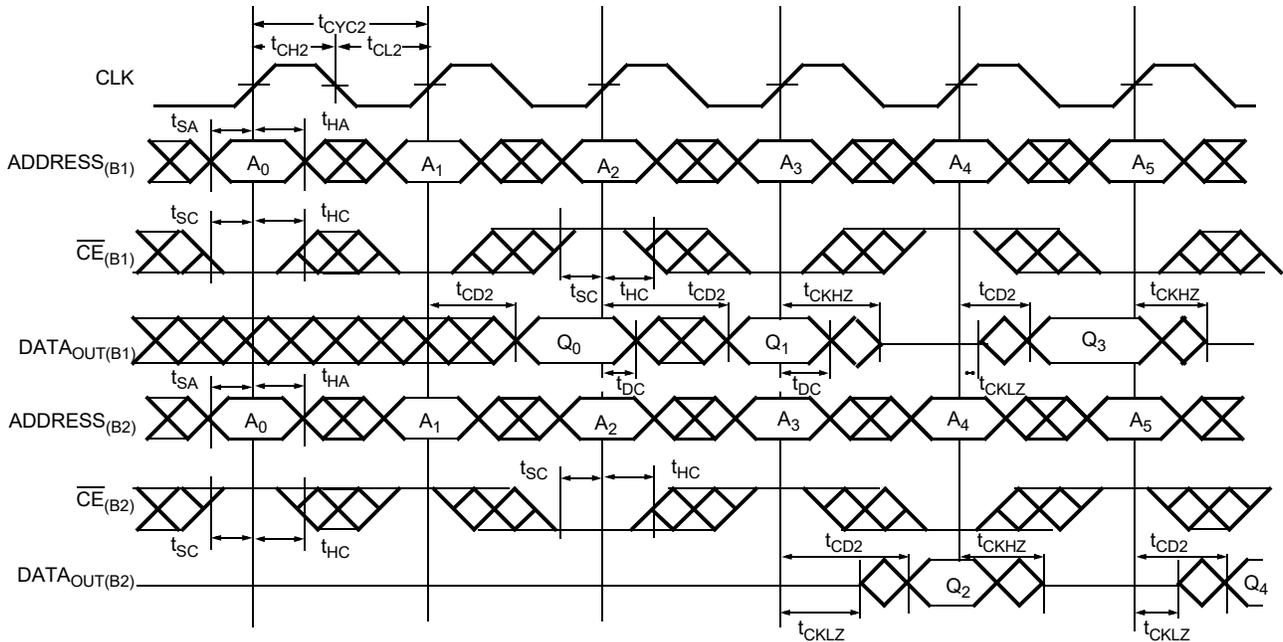
Figure 10. Read-to-Write-to-Read ( $\overline{OE} = \text{LOW}$ ) [36, 39, 40, 41, 42]
