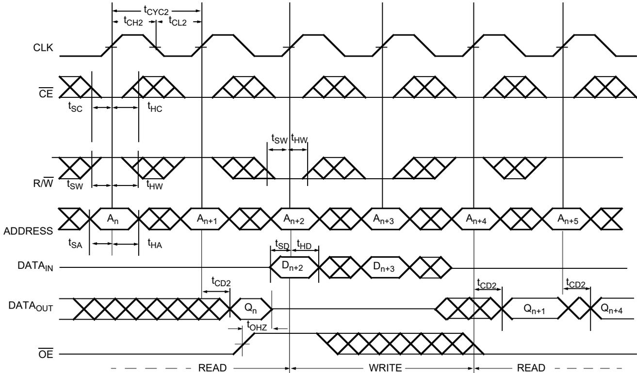
Figure 12. Read with Address Counter Advance [45]
