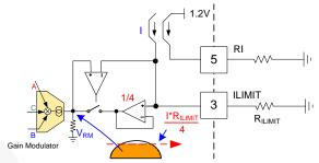
Figure 22. Current Command Limit by ILIMIT
