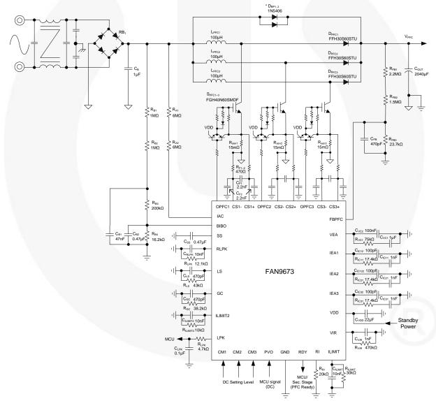
Figure 52. Schematic of Design Example
