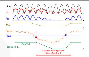
Figure 12. V<sub>VEA</sub> and V<sub>CM</sub> Relationship in Channel Management Operation
