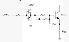
Figure 21. Gate Drive Circuit
