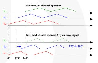
Figure 17. Phase Change under External Signal Control
