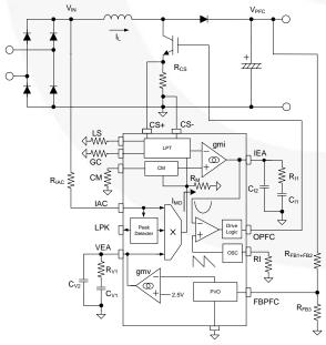
Figure 18. Gain Modulation Block
