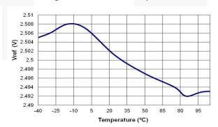
Figure 42. V<sub>PFC-OVP</sub> vs. Temperature
