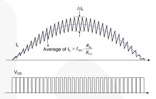
Figure 6. CCM PFC Operation Waveforms
