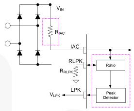
Figure 29. Relationship of V<sub>IN.PK</sub> to V<sub>LPK</sub>
