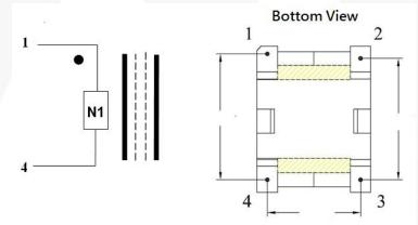
Figure 53. Inductor Schematic Diagram
