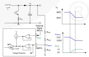
Figure 24. Programmable PFC Output Voltage
