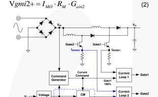
Figure 10. Channel Management / Gain Slave Channel Relationship
