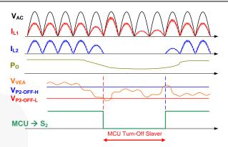
Figure 16. Channel Management by External Signal from MCU
