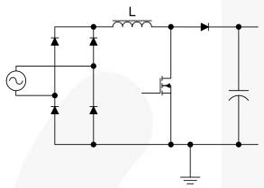
Figure 4. Basic PFC Boost Converter
