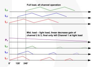
Figure 13. Phase and Gain Change of CM Control
