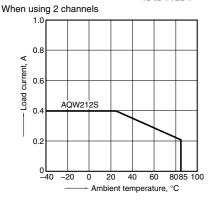
1.-(2) Load current vs. ambient temperature characteristics
