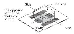
This power choke coil is different from the ferrite core-type that installs general concentration GAP. It has the leakage magnetic bunch distribution of the choke coil to the vertical direction. Please be cautious when using parts and circuit compositions which are easily affected by the leakage flux.
