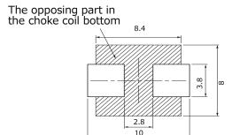
③Parts arranged around this power choke coil do not touch the surface of this power choke coil (Top side and side). (Series MC)
