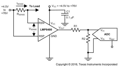
Figure 31. Typical Application With Resistive Divider Example
