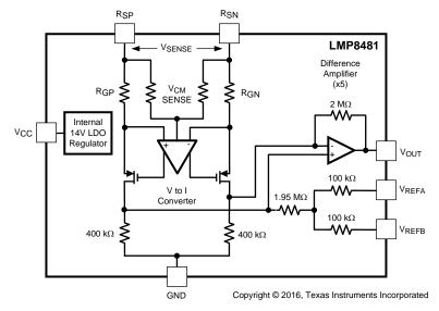
Figure 18. LMP8481 Block Diagram
