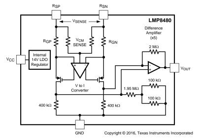
Figure 17. LMP8480 Block Diagram
