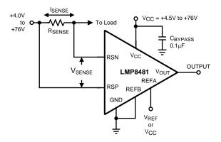
Figure 21. LMP8481 Basic Connections for Mid-Bias (V<sub>REF</sub> / 2) Input (Bidirectional)
