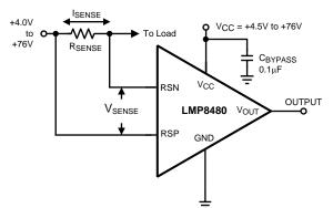
Figure 19. LMP8480 Basic Connections (Unidirectional)
