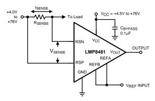
Figure 20. LMP8481 Basic Connections for External 1:1 V<sub>REF</sub> Input (Bidirectional)
