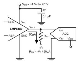
Figure 26. Output Pulldown Resistor Example
