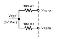
Figure 23. V<sub>REF</sub> Input Resistor Network
