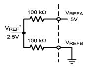
Figure 25. Applying a Divided Reference Voltage
