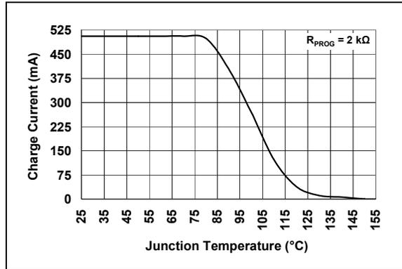
**FIGURE 2-10:** Charge Current ( $I_{OUT}$ ) vs. Junction Temperature ( $T_J$ ).
