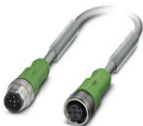
Sensor/actuator cable, 5-position, PUR halogen-free, highly flexible, gray RAL 7001, Plug straight M12, A-coded, on Socket straight M12, A-coded, cable length: 1 m
