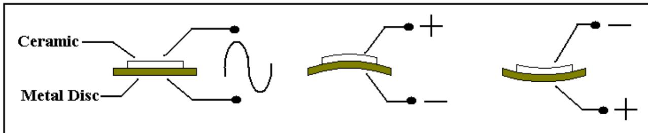
The above picture shows a bare piezoelectric sounder element. By applying a sinusoidal wave-form at an appropriate frequency, the transducer will physically deflect in one direction and then in the opposite direction following the shape of the input wave-form. If this oscillation occurs in the audible frequency range (1 Hz to 20 kHz), then air pressure waves are produced that the human ear interprets as an audible sound.
