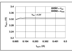
**FIGURE 2-12:** V<sub>OUT1</sub> vs. I<sub>OUT1</sub> (V<sub>OUT1</sub> = 3.3V).
