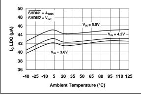
**FIGURE 2-3:** I<sub>Q</sub> LDO Current vs. Ambient Temperature.
