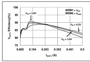
**FIGURE 2-7:**  $V_{OUT1}$  Output Efficiency vs.  $I_{OUT1}$  ( $V_{OUT1} = 1.8V$ ).
