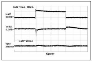
FIGURE 2-32: V<sub>OUT2</sub> Load Step Response vs. Time.
