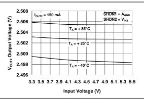
**FIGURE 2-23:**  $V_{OUT2}$  Output Voltage vs. Input Voltage ( $V_{OUT2} = 2.5V$ ).
