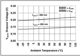
FIGURE 2-25: V<sub>OUT2</sub> Dropout Voltage vs. Ambient Temperature ( $V_{OUT2} = 2.5V$ ).
