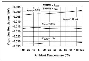
**FIGURE 2-27:** V<sub>OUT2</sub> Line Regulation vs. Ambient Temperature.
