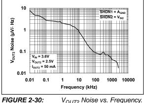
V<sub>OUT2</sub> Noise vs. Frequency.
