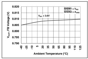
FIGURE 2-15: V<sub>OUT1</sub> Adjustable Feedback Voltage vs. Ambient Temperature.
