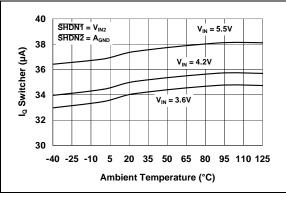
**FIGURE 2-2:** I<sub>Q</sub> Switcher Current vs. Ambient Temperature.
