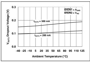
FIGURE 2-26: V<sub>OUT2</sub> Dropout Voltage vs. Ambient Temperature ( $V_{OUT2} = 3.3V$ ).
