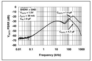
FIGURE 2-29: V<sub>OUT2</sub> Power Supply Ripple Rejection vs. Frequency.
