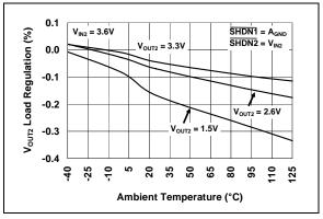
FIGURE 2-28: V<sub>OUT2</sub> Load Regulation vs. Ambient Temperature.
