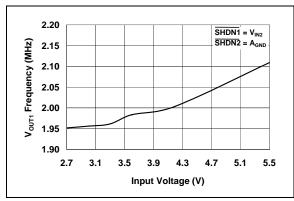
FIGURE 2-13: V<sub>OUT1</sub> Switching Frequency vs. Input Voltage.
