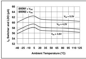
**FIGURE 2-1:** I<sub>Q</sub> Switcher and LDO Current vs. Ambient Temperature.
