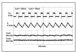
*FIGURE 2-19:* V<sub>OUT1</sub> and V<sub>OUT2</sub> Heavy Load Switching Waveforms vs. Time.
