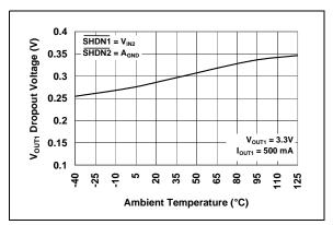
**FIGURE 2-18:** V<sub>OUT1</sub> Dropout Voltage vs. Ambient Temperature.
