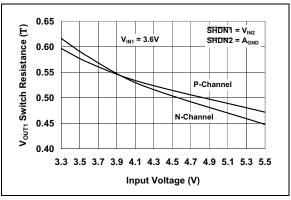
*FIGURE 2-16:* V<sub>OUT1</sub> Switch Resistance vs. Input Voltage.
