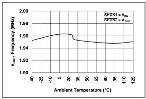
**FIGURE 2-14:** V<sub>OUT1</sub> Switching Frequency vs. Ambient Temperature.
