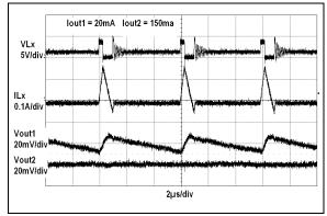
**FIGURE 2-20:** V<sub>OUT1</sub> and V<sub>OUT2</sub> Light Load Switching Waveforms vs. Time.
