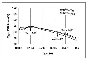
**FIGURE 2-5:**  $V_{OUT1}$  Output Efficiency vs.  $I_{OUT1}$  ( $V_{OUT1} = 1.2V$ ).
