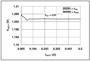
**FIGURE 2-10:** V<sub>OUT1</sub> vs. I<sub>OUT1</sub> (V<sub>OUT1</sub> = 1.2V).
