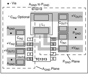
FIGURE 5-1: Component Placement, Fixed-Output 10-Pin MSOP.
