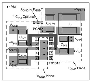
FIGURE 5-2: Component Placement, Fixed-Output 10-Pin DFN.
