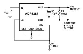
Figure 11. Dropout Status Output
