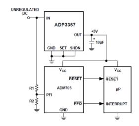
Figure 15. μP Regulator with Supply Monitoring and Early Power-Fail Warning
