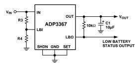
Figure 10. Low Battery/Supply Detect Circuit
