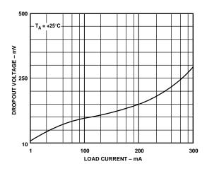
Figure 2. Dropout Voltage vs. Load Current
