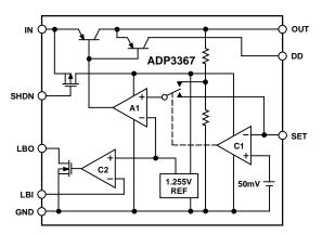
Figure 1. ADP3367 Functional Block Diagram
