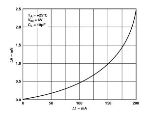
Figure 5. Load Regulation (DV $_{OUT}$  vs. DI $_{OUT}$ )
