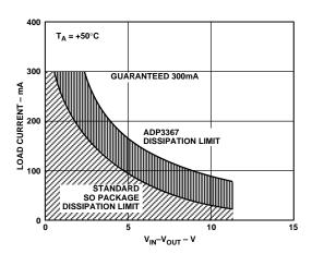
Load Current vs. Input-Output Differential Voltage
