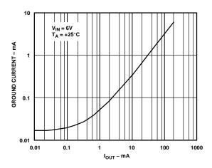
Figure 3. Ground Current vs. Load Current
