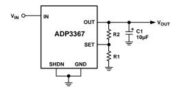
Figure 9. Adjustable Output Circuit
