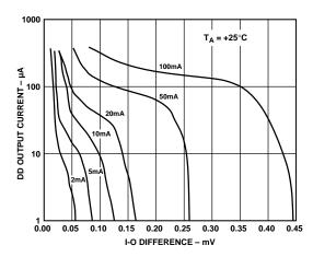
Figure 4. DD Output Current vs. I-O Differential
