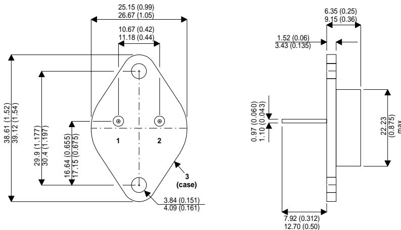
**Bipolar NPN Device in a
