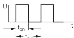
$$df = \frac{t_{on}}{t_{cyc}} \times 100 \text{ (%)}$$
