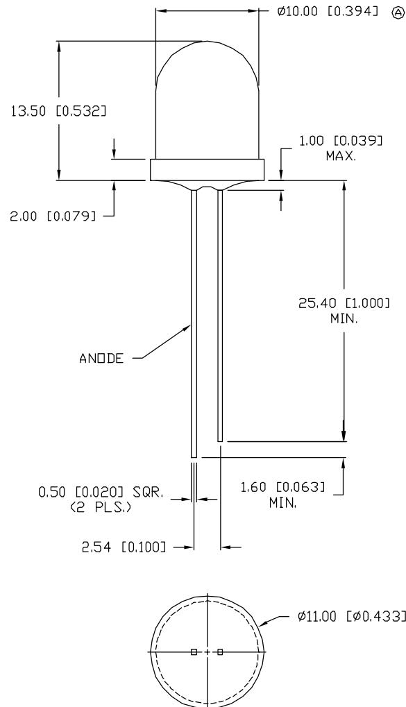
UNLESS OTHERWISE SPECIFIED TOLERANCE IS  $\pm 0.25\text{mm}$  ( $\pm 0.010$ )ELECTRO-OPTICAL CHARACTERISTICS  $T_A = 25^\circ\text{C}$   $I_f = 20\text{mA}$
