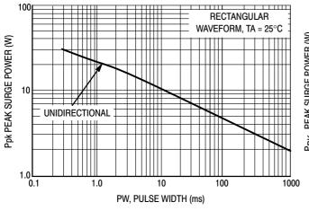
Figure 7. Maximum Non-Repetitive Surge Power, P<sub>pk</sub> versus PW
