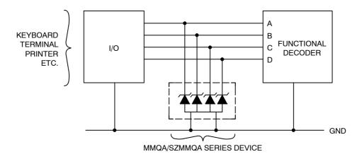
Figure 9. Computer Interface Protection
