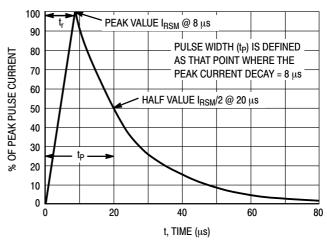
Figure 6.  $8 \times 20~\mu s$  Pulse Waveform
