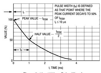
Figure 5. 10  $\times$  1000  $\mu s$  Pulse Waveform
