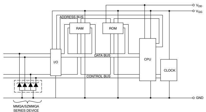
Figure 10. Microprocessor Protection
