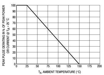
Figure 3. Steady State Power Derating Curve
