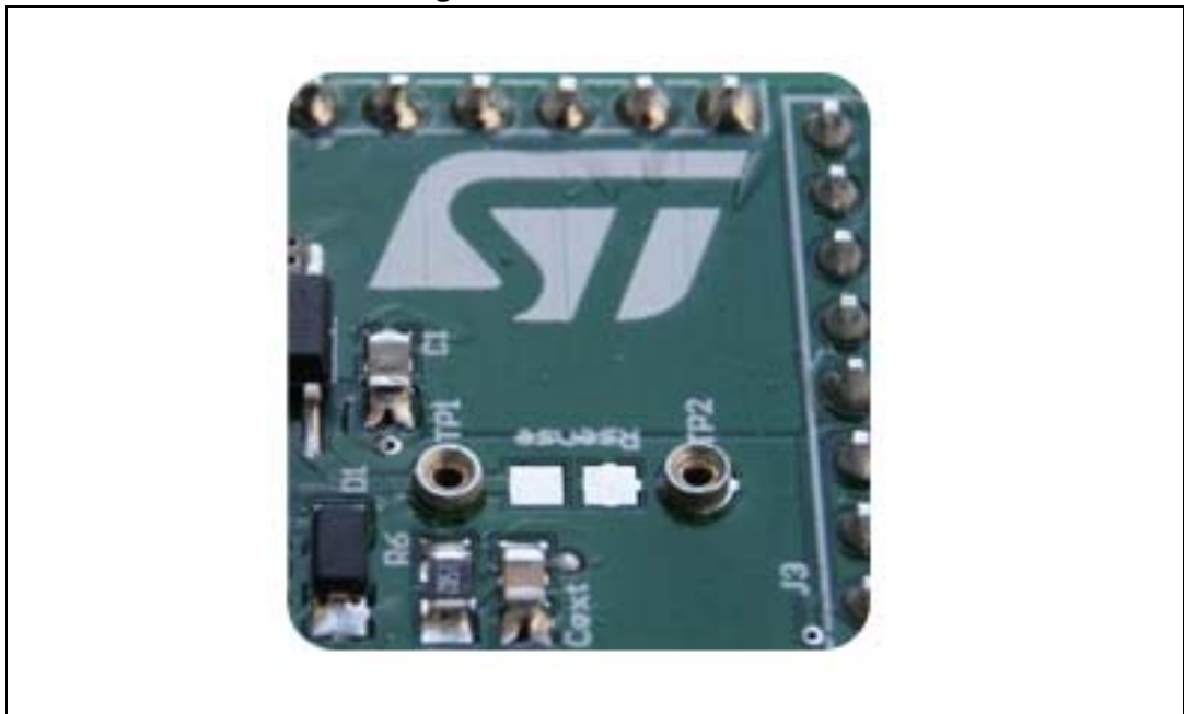
Figure 4. Mounting through-hole sense resistor
