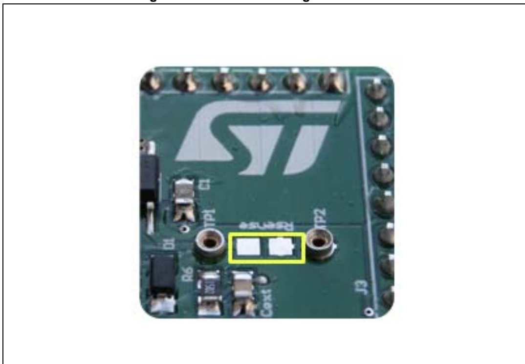
Figure 5. Pads for soldering SMD resistor
