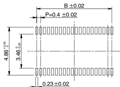
Recommended solder paste thickness: 120  $\mu\text{m}$
