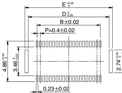
Recommended solder paste thickness: 120  $\mu$ m
