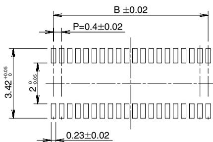
Recommended solder paste thickness: 120 μm
