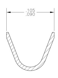
SECTION B-B INSULATION RANGE .025–.060 SCALE 20:1
