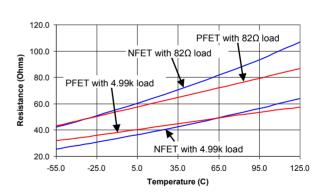
6. Output resistance were measured under the condition of  $V_{CC}$  = +5.0 V,  $V_{OPT}$  = +5.0 V, and  $V_{EE}$  = -5.0 V, with load resistors from outputs to ground.
