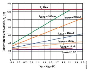
Figure 31. 100 mm<sup>2</sup> of PCB Copper,  $T_A = 25$ °C
