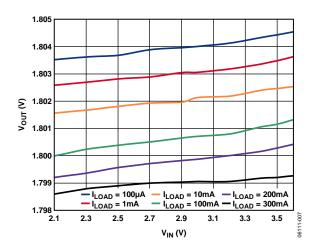
Figure 5. Output Voltage vs. Input Voltage
