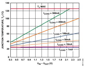
Figure 30. 500 mm<sup>2</sup> of PCB Copper,  $T_A = 25^{\circ}$ C
