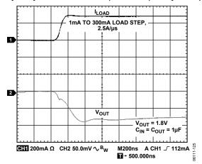
Figure 24. Output Transient Response,  $C_{OUT} = 1 \mu F$
