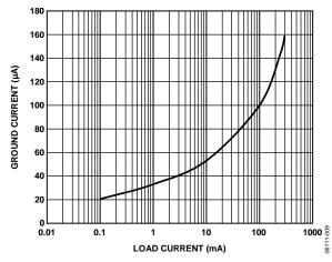
Figure 7. Ground Current vs. Load Current
