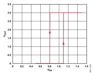
Figure 27. ADP172 Typical EN Pin Operation
