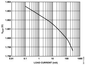
Figure 4. Output Voltage vs. Load Current
