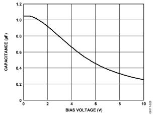
Figure 26. Capacitance vs. Bias Voltage Characteristics
