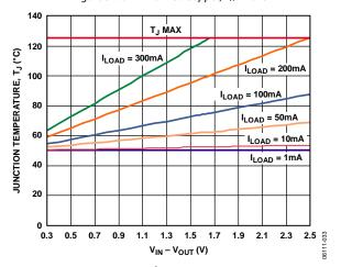
Figure 33. 500 mm<sup>2</sup> of PCB Copper,  $T_A = 50$ °C
