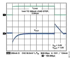
Figure 19. Load Transient Response,  $C_{IN}$  and  $C_{OUT} = 1 \mu F$
