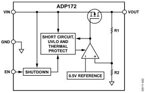
Figure 23. ADP172 Internal Block Diagram
