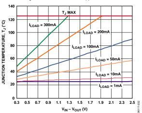
Figure 32. 0 mm<sup>2</sup> of PCB Copper,  $T_A = 25$ °C
