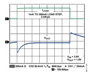
Figure 20. Load Transient Response,  $C_{IN}$  and  $C_{OUT} = 4.7 \mu F$
