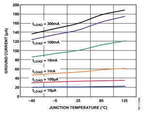
Figure 6. Ground Current vs. Junction Temperature
