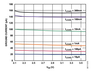
Figure 8. Ground Current vs. Input Voltage
