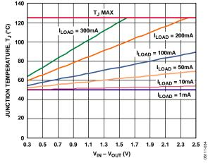
Figure 34. 100 mm<sup>2</sup> of PCB Copper,  $T_A = 50$ °C
