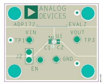
Figure 37. Example ADP172 PCB Layout
