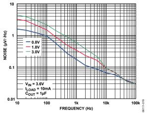
Figure 17. Output Noise Spectrum
