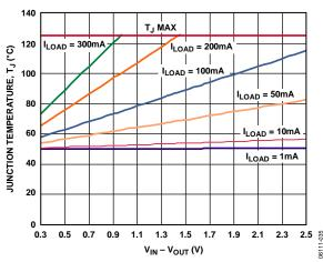
Figure 35. 0 mm<sup>2</sup> of PCB Copper,  $T_A = 50^{\circ}$ C
