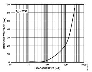
Figure 10. Dropout Voltage vs. Load Current
