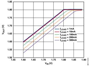
Figure 11. Output Voltage vs. Input Voltage (in Dropout)
