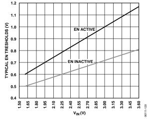
Figure 28. Typical EN Pin Thresholds vs. Input Voltage
