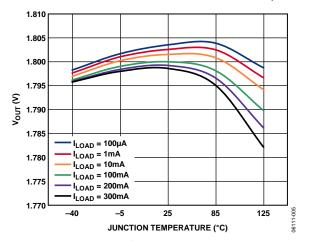
Figure 3. Output Voltage vs. Junction Temperature
