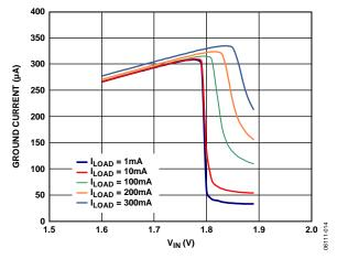
Figure 12. Ground Current vs. Input Voltage (in Dropout)
