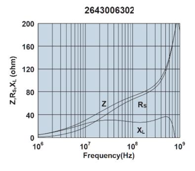
Impedance, reactance, and resistance vs. frequency.
