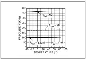
**FIGURE 2-13:** EL Frequency vs. Temperature.
