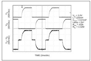
FIGURE 4-1: 108 Hz Typical Output Waveform.
