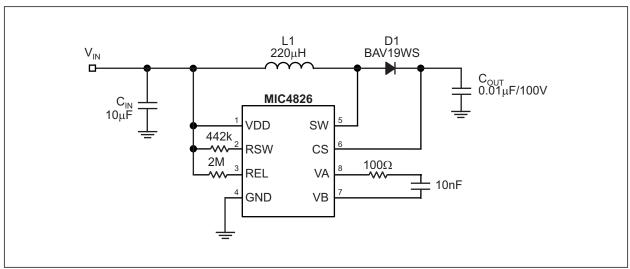
FIGURE 1-1: MIC4826 Test Circuit.
