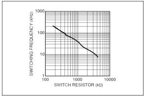
FIGURE 2-8: Switch Resistor.
