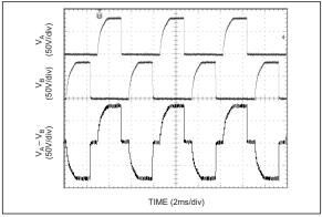
FIGURE 4-2: 180 Hz Output Waveform.
