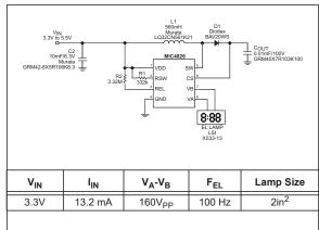
**FIGURE 5-5:** EL Driver for  $2in^2$  Lamp with 560  $\mu$ F.
