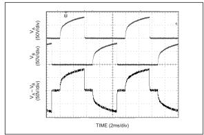
FIGURE 5-6: Typical Characteristics for EL Driver for 2in<sup>2</sup> Lamp with 560 μH Inductor.
