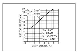
**FIGURE 2-15:** Total Input Current vs. Lamp Size.
