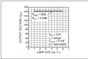
FIGURE 2-14: Output Voltage vs. Lamp Size.
