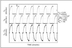
FIGURE 4-3: 360 Hz Output Waveform.
