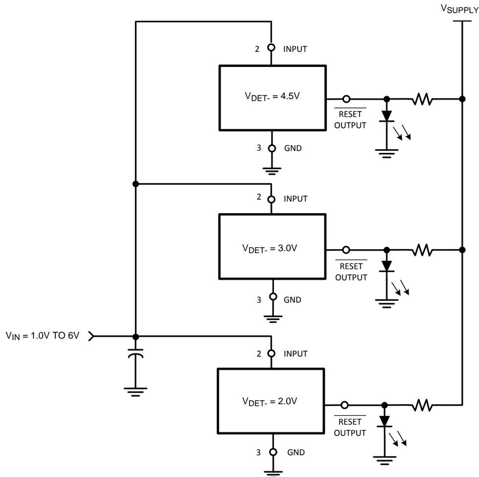
EACH LED WILL SEQUENTIALLY TURN ON WHEN THE RESPECTIVE VOLTAGE DETECTOR THRESHOLD ( $V_{DET-} + V_{HYS}$ ) IS EXCEEDED.
