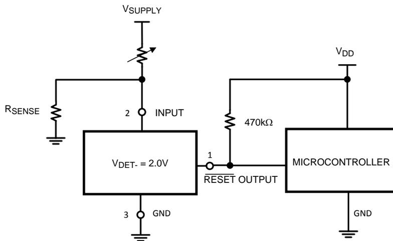
THIS CIRCUIT MONITORS THE CURRENT AT THE LOAD. AS CURRENT FLOW THROUGH THE LOAD, A VOLTAGE DROP WITH RESPECT TO GROUND APPEARS ACROSS  $R_{SENSE}$  WHERE  $V_{SENSE} = I_{LOAD} * R_{SENSE}$ . THE FOLLOWING CONDITIONS APPLY:
