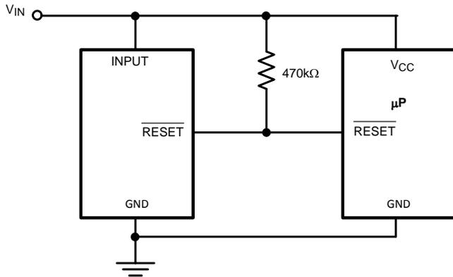
Figure 9. Microprocessor Reset Circuit
