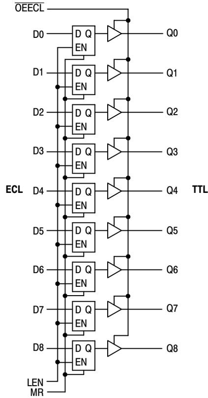
Figure 2. Logic Diagram
