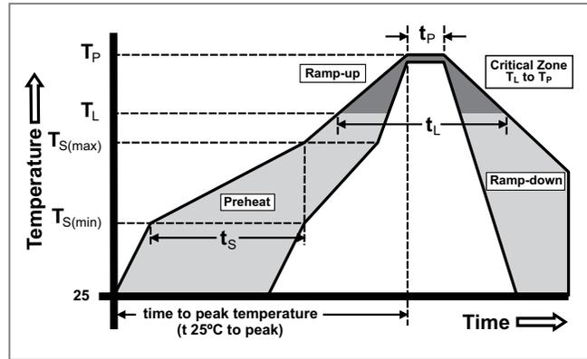
**Soldering Parameters - Wave Soldering (Thru-Hole Devices)**
